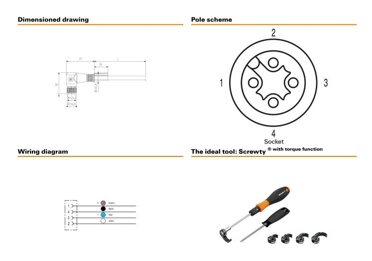
Light, securely screwed-in round plug-in connectors. Screwty set DM / VPE: 1 / Order No.: 1920000000 Adapters: M12, M12 F, M8, M8 F
