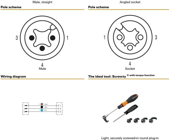
connectors. Screwty set DM / VPE: 1 / Order No.: 1920000000 Adapters: M12, M12 F, M8, M8 F
