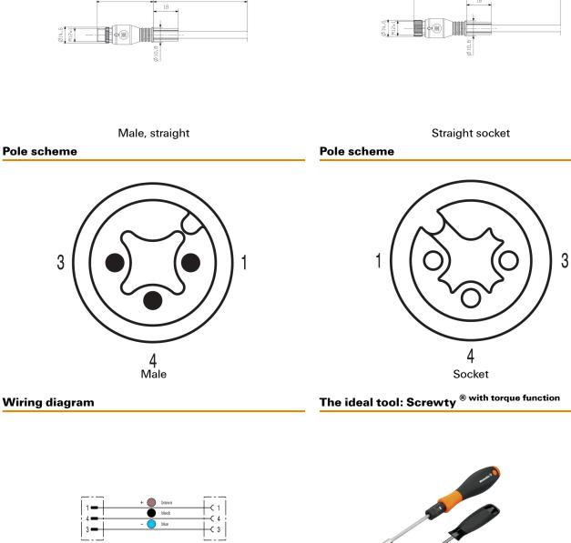
Light, securely screwed-in round plug-in connectors. Screwty set DM / VPE: 1 / Order No.: 192000000 Adapters: M12, M12 F, M8, M8 F
