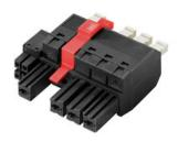
180° female plug with energy and signal contacts in PUSH IN wire connection in 7.62 pitch. Fulfils the IEC 61800-5-1 requirement and for the energy contact UL 1059 ClassC 600 V. With adjustable, self-locking pusher for opening the contact point.
