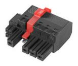
180° female plug with energy and signal contacts in PUSH IN wire connection in 7.62 pitch. Fulfils the IEC 61800-5-1 requirement and for the energy contact UL 1059 ClassC 600 V.
