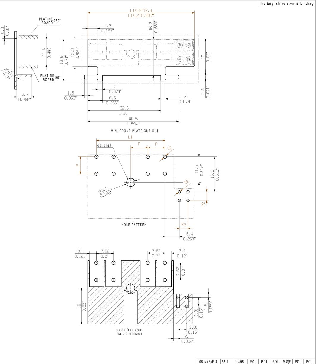
$D1 = \emptyset 1.4 + 0.1/-0.05$   $D2 = \emptyset 1.2 + 0.1/-0.05$  d = 0.8x1.0 P = Raster/pitch 7.62 P2 = Raster/pitch 3.81 MF = Mittelflansch middle flangeMittelseberuch flange h
