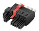
180° female plug with energy and signal contacts in PUSH IN wire connection in 7.62 pitch. Fulfils the IEC 61800-5-1 requirement and for the energy contact UL 1059 ClassC 600 V. With adjustable, self-locking pusher for opening the contact point.
