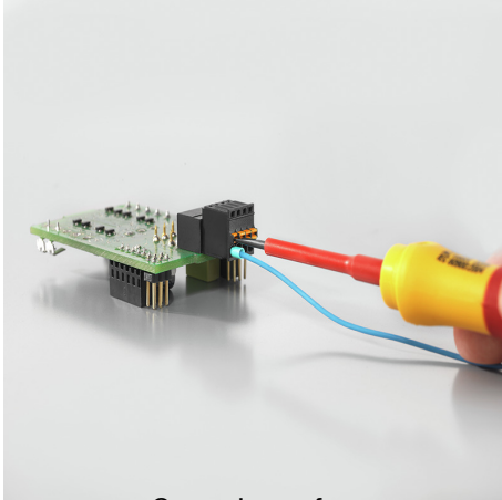
Operating safety Through PUSH IN connection system
