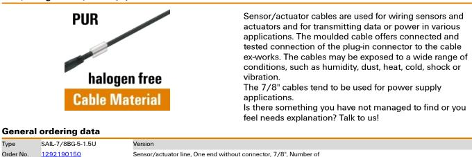
poles : 5 (4 + PE), 1.5 m, Female socket, straight, Shielded: No, LED:
