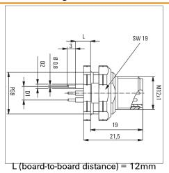
Front panel section D1 = 5,5 mm
