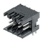
High-temperature-resistant, straight, 2-tier pin header for all common soldering methods. Optimized for automatic assembly. Packed in box or tape. 3.2 mm solder pin suitable for reflow and wave soldering. These pin headers can be labelled and coded. (Packaging in tape on request)
