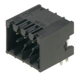
High-temperature-resistant, straight, 2-tier male connector for all common soldering methods. Optimised for automatic assembly. Packed in box or tape. 3.2 mm solder pin suitable for reflow and wave soldering. These male connectors can be labelled and coded.
