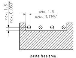
D= 1.4/0.055" or 1.5/0.059"(REFLOW SOLDERING) RECOMMENDATION FOR AUTOMATIC ASSEMBLY (1.4mm FOR n=2...8 / 1.5mm for n=9...24)
