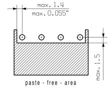
D = 1.4/0.055" or 1.5/0.059" (REFLOW SOLDERING) RECOMMENDATION FOR AUTOMATIC ASSEMBLY (1.4 mm FOR n = 2...8 / 1.5 mm for n = 9...24)
