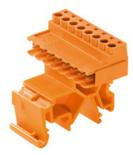
Male plugs with clamping-yoke screw wire-connect system. With clip-on feet for attaching the male plugs on rail. The male plugs provide space for labelling and can be coded.
