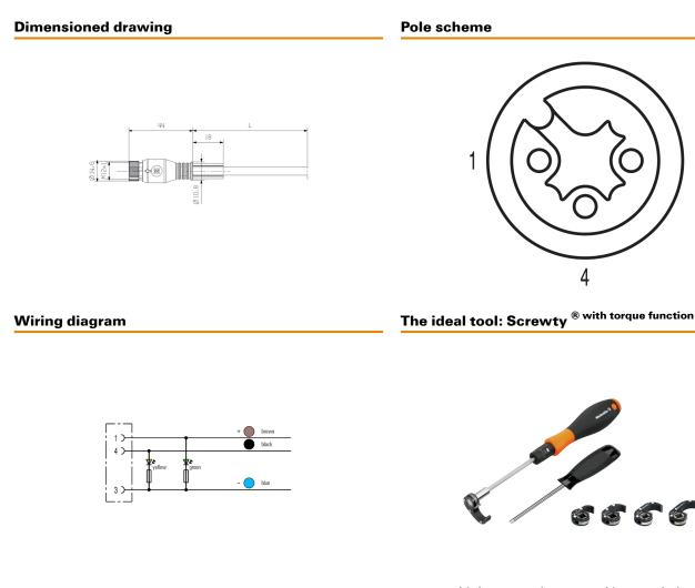
Light, securely screwed-in round plug-in connectors. Screwty set DM / VPE: 1 / Order No.: 192000000 Adapters: M12, M12 F, M8, M8 F
