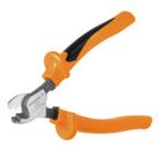
Cutting tools for conductors up to 8 mm, 12 mm, 14 mm and 22 mm outside diameter. The special blade geometry allows pinch-free cutting of copper and aluminium conductors with minimum physical effort. The cutting tools also come with VDE and GS-tested protective insulation up to 1,000 V in accordance with EN/IEC 60900.
