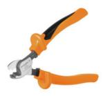
Cutting tools for conductors up to 8 mm, 12 mm, 14 mm and 22 mm outside diameter. The special blade geometry allows pinch-free cutting of copper and aluminium conductors with minimum physical effort. The cutting tools also come with VDE and GS-tested protective insulation up to 1,000 V in accordance with EN/IEC 60900.
