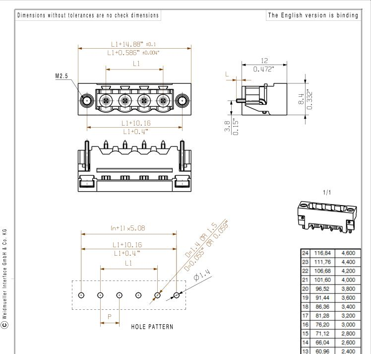
For the mounting of PCBs, it should be noted that the rated data given in the catalogue relates only to the connection elements. The neccessary creepage and clearance paths must be observed in connection with the respective applicant in accordance to VDE 0110. The current-carrying capacity and pitch tolerance is to be determined according to IEC 60326 part 3 very fine.
