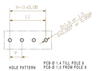
For the mounting of PCBs, it should be noted that the rated data given in the catalogue relates only to the connection elements. The neccessary creepage and clearance paths must be observed in connection with the respective applicant in accordance to VDE 0110. The current-carrying capacity and pitch tolerance is to be determined according to IEC 60326 part 3 very fine.
