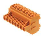
Female plugs with two clamping-yoke screw connections per pole for wire connections with 90° and 270° outlet directions. The female plugs provide space for labelling and can be coded.
