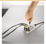
Tools for stripping the sheathing from uncut power lines and outlet lines, plus screwdrivers for installing Pick-to-Light components.
