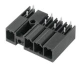
270° male header with middle flange with a 7.62 pitch. Meets the requirements of IEC 61800-5-1 and enables UL approval as per UL840 600 V. Without a female header, the mating profile guarantees minimum touch safety of >3 mm with 20 N pressure on the test finger. The automatically locking middle flange which can optionally also be screwed, reduces space requirements by one pitch width in comparison with conventional solutions.
