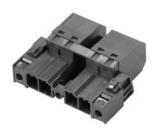
180° inverted male header with PUSH IN connection technology for field wiring in 6 mm² with 7.62 pitch as "three-flange variant" for housing passage. Suitable for housings with a max. wall thickness of 2 mm. Also perfect as a finger-safe solution for inverse voltages. Meets the requirements of UL1059 600 V class C and IEC 61800-5-1.
