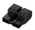
180° inverted inverse voltage-safe male header with PUSH IN connection technology for field wiring. With automatically locking middle flange for field wiring in 6 mm² with 7.62 pitch.
