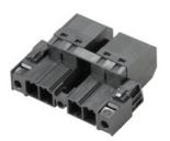
180° inverted male header with PUSH IN connection technology for field wiring in 6 mm² with 7.62 pitch as "three-flange variant" for housing passage. Suitable for housings with a max. wall thickness of 2 mm. Also perfect as a finger-safe solution for inverse voltages. Meets the requirements of UL1059 600 V class C and IEC 61800-5-1.
