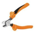
Cutting tools for conductors up to 8 mm, 12 mm, 14 mm and 22 mm outside diameter. The special blade geometry allows pinch-free cutting of copper and aluminium conductors with minimum physical effort. The cutting tools also come with VDE and GS-tested protective insulation up to 1,000 V in accordance with EN/IEC 60900.
