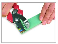
Cut off insulation via cutter.
