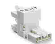
Item no.890-980 h-distribution connector; 5-pole; Cod. A; 1 input; 2 outputs; outputs on one side; 3 locking levers; for flying leads; white
