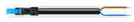
Item no.891-8982/206-101 pre-assembled connecting cable; Eca; Plug/open-ended; 2-pole; Cod. I; H05VV-F 2 x 1.5 mm 2 ; 1 m; 1,50 mm 2 ; blue
