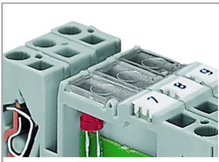
Marking using miniature WSB quick marking card
