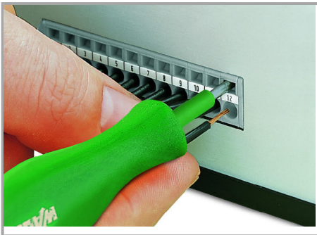
Feedthrough PCB terminal strips – front-entry conductor termination
