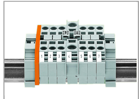
Commoning from 10 mm 2 /8 AWG (284 Series) to 6 mm 2 /10 AWG (282 Series) rail-mount terminal blocks via step-down jumpers.
