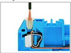
Insert stripped, untwisted conductor into insulation stop.
