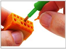
Sealing unnecessary clamping points in CAGE CLAMP®-equipped male and female connectors (e.g., when doubling the pin spacing to meet clearance and creepage distance requirements, or when higher rated voltage is required). Lockout pins are not suitable for panel-mount, angled female connectors.
