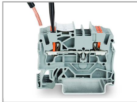
Insert fine-stranded conductors via operating tool.
