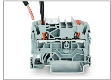
Insert fine-stranded conductors via operating tool.
