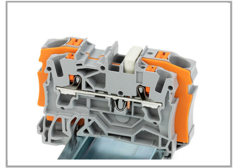
Step-down jumper (2006-499) commons 6 /4 mm 2 (10/12 AWG) terminal blocks (2206 /2204 Series) with 4/2.5/1.5 mm 2 (12/14/16 AWG) terminal blocks (2204/2202/2201 Series).
