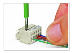
Inserting a conductor via  $(2.5 \times 0.4)$  mm screwdriver. Operation is performed perpendicular to conductor entry.
