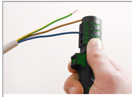
Stripping a wire insulation.
