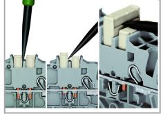
Removing a push-in type jumper bar.
