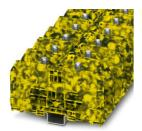
Bolt connection terminal block, nom. voltage: 1000 V, nominal current: 309 A, number of connections: 2, number of positions: 1, connection method: Bolt connection, 1 level, Rated cross section: 150 mm<sup>2</sup>, mounting type: NS 35/7,5, NS 35/15, direct screw connection, color: black/yellow
