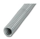
Protective hose, material: PVC, filament: PVC sheathed spring steel, UV-resistant: no, flexible, degree of protection: IP68, color: gray, inner diameter: 29 mm, Total length: 10 m
