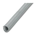
Protective hose, material: PVC, filament: PVC sheathed spring steel, UV-resistant: no, flexible, degree of protection: IP68, color: gray, inner diameter: 22 mm, Total length: 10 m
