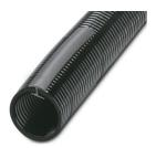
Protective hose, material: PA, UV-resistant: yes, flexible, degree of protection: IP40, color: black, flammability rating in acc. with UL 94: HB, inner diameter: 29 mm, Total length: 10 m
