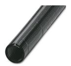
Protective hose, material: PA, UV-resistant: yes, flexible, degree of protection: IP40, color: black, flammability rating in acc. with UL 94: HB, inner diameter: 23 mm, Total length: 10 m
