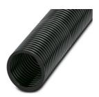
Protective hose, material: PA 6, UV-resistant: yes, flexible, degree of protection: IP68, color: black, flammability rating in acc. with UL 94: HB, inner diameter: 36 mm, Total length: 25 m
