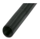
Protective hose, material: PA 6, UV-resistant: yes, flexible, degree of protection: IP68, color: black, flammability rating in acc. with UL 94: HB, inner diameter: 23 mm, Total length: 50 m
