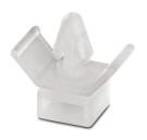
Cable binder base, for cable binders of up to 8 mm, with molded body-bound rivet, 6.5 mm drilling diameter, for material thicknesses up to 3 mm
