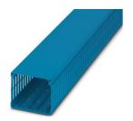
Cable duct for installation and mounting in control cabinets, blue, comprising upper part and mounting base, width: 100 mm, height: 80 mm, length: 2000 mm
