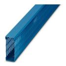
Cable duct for installation and mounting in control cabinets, blue, comprising upper part and mounting base, width: 40 mm, height: 100 mm, length: 2000 mm
