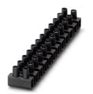
Polypropylene Europe terminal strip, black, for connecting solid conductors and stranded conductors with and without ferrules with a cross section of 1.5 to 16 mm<sup>2</sup>
