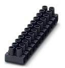
Polypropylene Europe terminal strip, black, for connecting solid conductors and stranded conductors with and without ferrules with a cross section of 0.5 to 4 mm<sup>2</sup>
